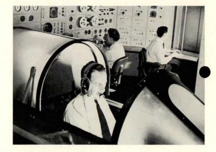
The F-89D Simulator in operation shows pilot, concentrating on his instrument panel, with radar instructor, upper left, and flight instructor checking and controlling the entire flight problem.
